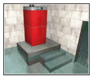
Example of raising the height of sensitive installations above flood water level
